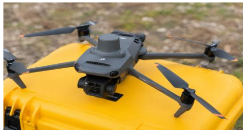
Figure 2. DJI Mavic 3 RTK UAV used during data acquisition.
