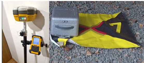
Figure 3. HI-TARGET V30 GNSS receiver and Ground Control Point used during the survey.
