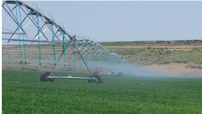
Fig. 7. Pivot irrigation system implemented at the agricultural unit – Agro Mares SRL (original photo)
