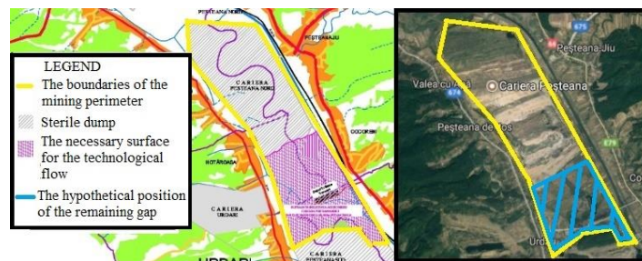
Figure 3. The boundaries of North Peșteana mining perimeter and the final (hypothetical) position of the remaining gap
