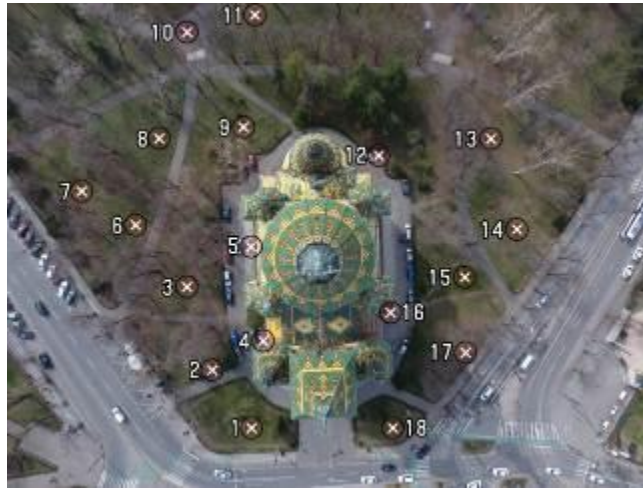
Figure 7 - Ground points used for georeference
