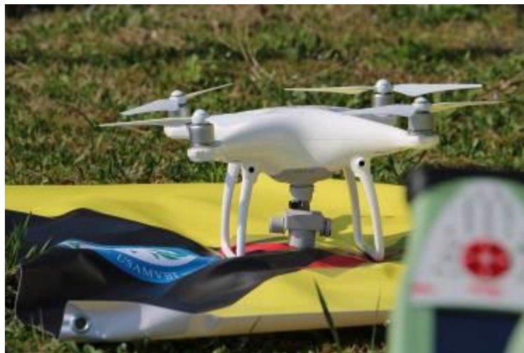
Figure 4 - UAV Phantom4 Pro together with the Leica GS058
