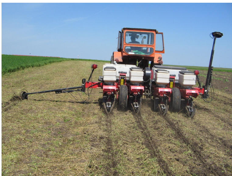
Fig. 1. Trial device for the study of the dynamics and energy of the direct sowing unit
