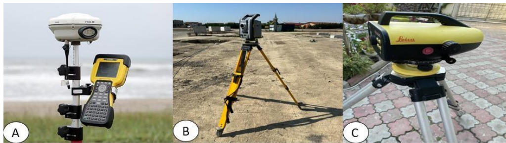
Fig. 1 a – R8 gnss survey, b – Trimble s7 total station, c – Leica sprinter 250m
