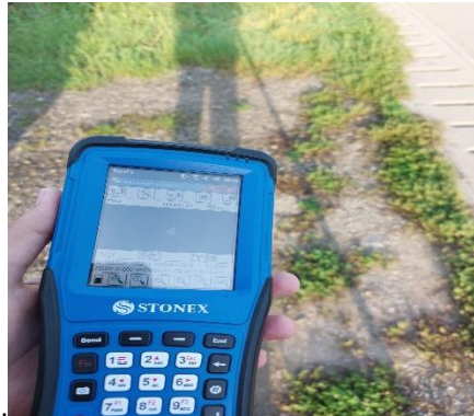
Fig.4 GPS Stonex S10 during use, for making the geodetic network
