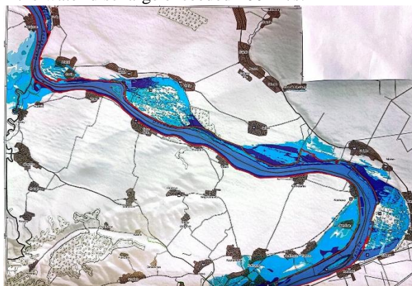
Figure 7. Flood Hazard Map for the Gruia – Basarabi Sector.
