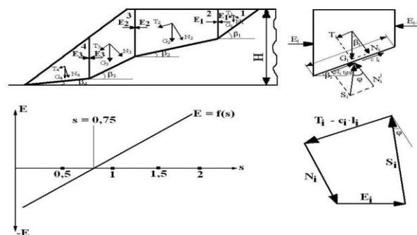
Figure 5. Stability analysis for polygonal surfaces (ROTUNJANU, 2005; LAZĂR ET FAUR, 2015)
