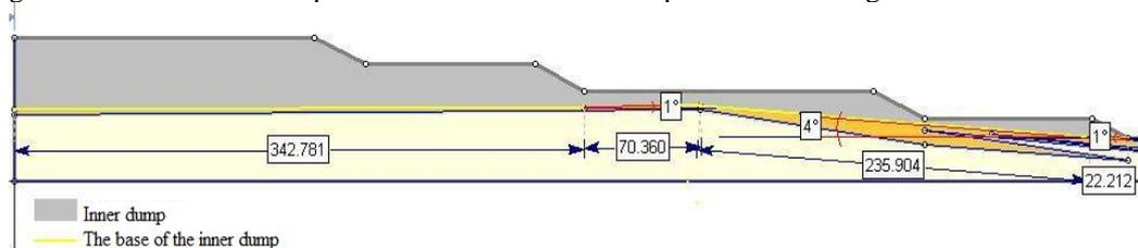
Figure 3. The base of the inner dump - geometrical characteristics (APOSTU, 2018)
