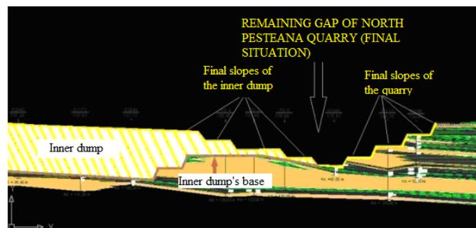
Figure 2. Longitudinal section - the remaining gap of North Pesteana quarry (APOSTU, 2018)
