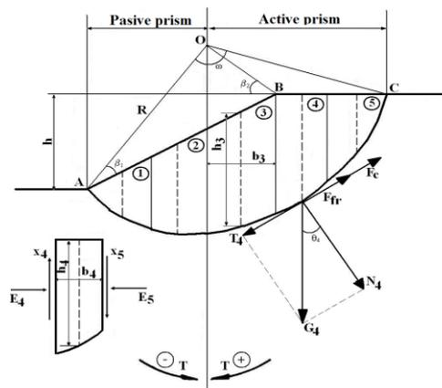
Figure 4. Calculation principle of the stability coefficient using the Fellenius method (ROTUNJANU, 2005; LAZĂR ET FAUR, 2015)
