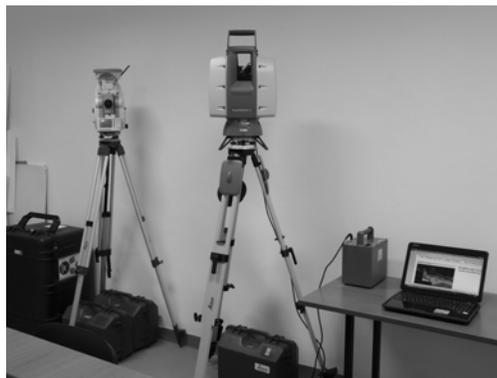
Figure 6: Laser Scanner 3D - HDS Leica Geosystems
