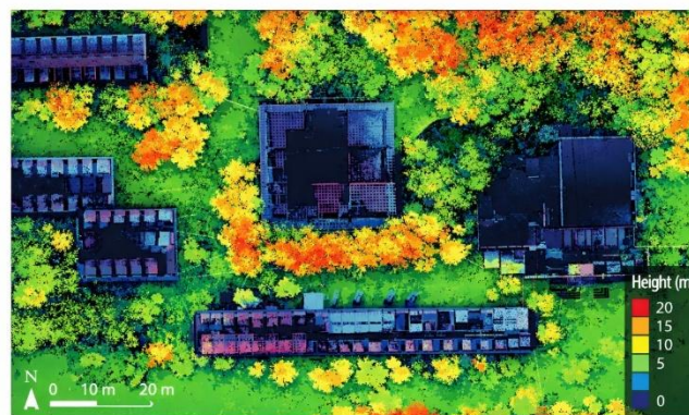
Figure 7. Point cloud coloured by elevation illustrating the differentiation between buildings and vegetation, USV Timisoara
