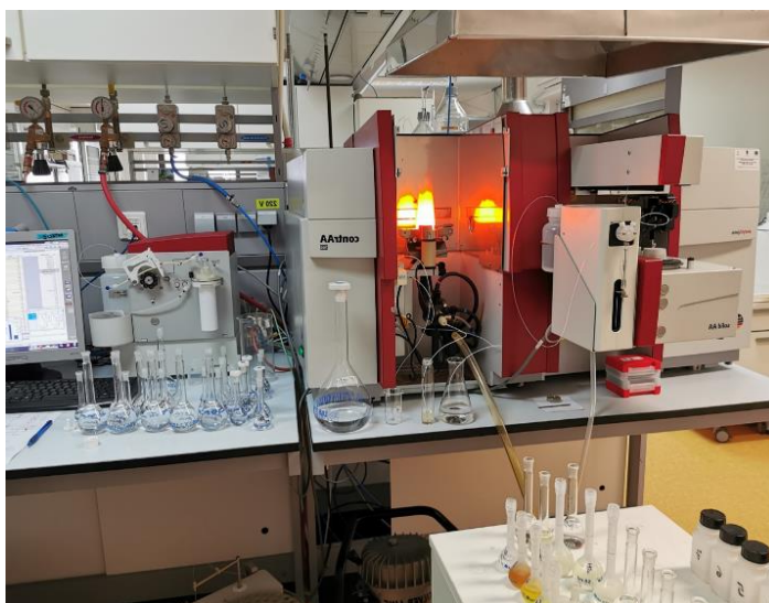
Figure 4 - Atomic absorption spectrometry with a flame atomizer system
