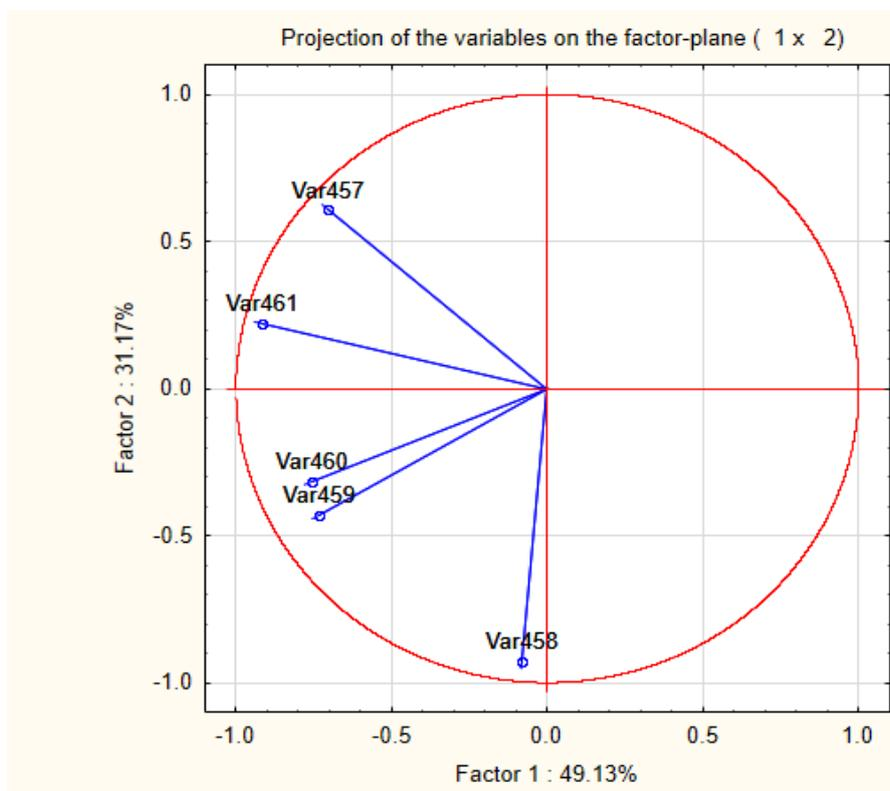
**Var 457** – Cu concentration - experimental site 1, mg/kg; **Var 458** – Zn concentration - experimental site 2, mg/kg; **Var 459** – Pb concentration - experimental site 3, mg/kg; **Var 460** – Cd concentration - experimental site 4, mg/kg; **Var 461** – Ni concentration - experimental site 5, mg/kg;
