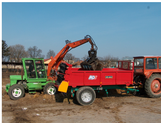
Fig.2. Operating mode of the grab bucket loader arrangement
