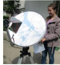
Figure 10. Solar generator with parabolic concentrator
