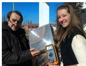
Figure 7. Solar generator with Fresnel lens and thermoelectric module
