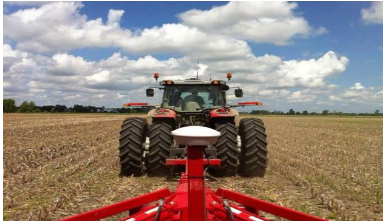
Figure 4. GPS antenna on the tractor trailer
