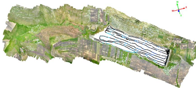
Figure 4. Cătămărăști accumulation point cloud - studied area, bottom of the lake, dam body
