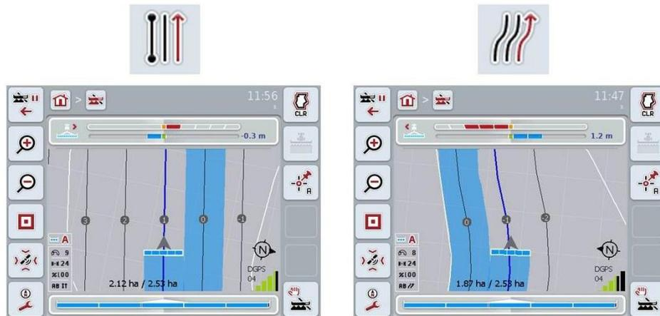
Figure 3 Parallel Tracking straight and curve mode
