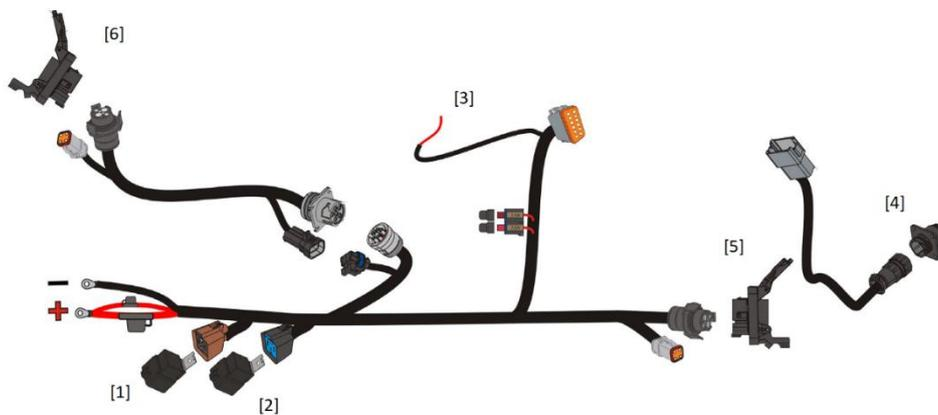
Figure 1. ISOBUS connectors and wire harness
