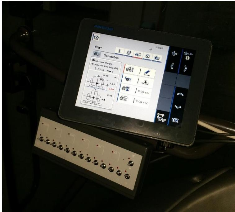
Figure 2. ANEDO open panel T50i terminal and ANEDO open ISOBUS box with switches
