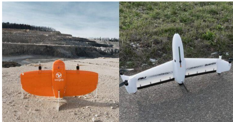
Fig. 3 - Comparison of two best VTOL aircraft for topography
