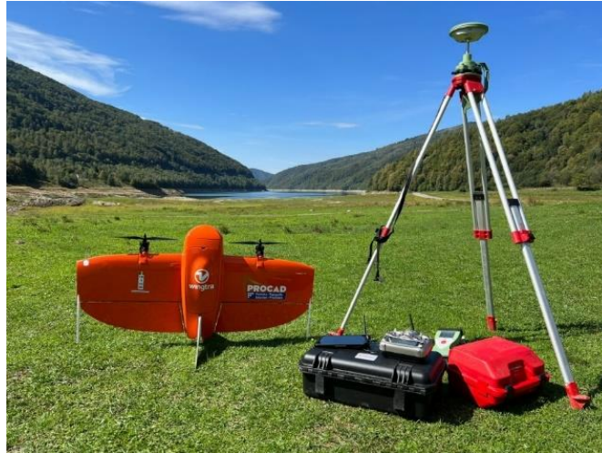
Fig. 2 - WingtraOne Generation II, UAT Zavoi, Poiana Mărului, Caras-Severin, the use of this technology brought to the realization of the orthophotoplane in the studied area.
