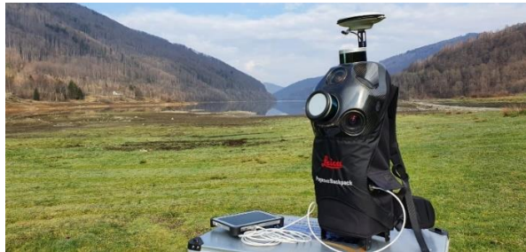
Fig. 4 - Equipment Leica Pegasus Backpack, Zăvoi Commune
