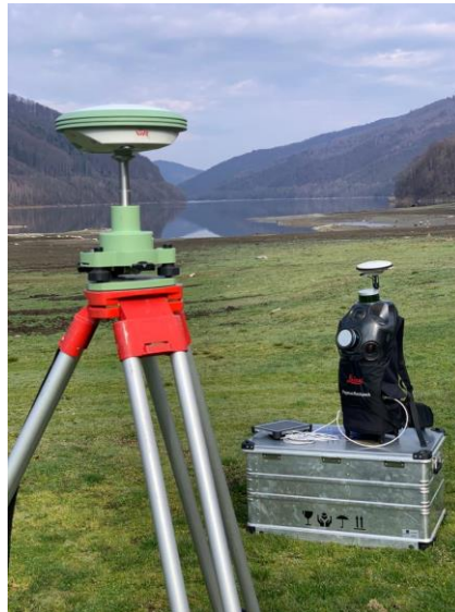
Fig. 5 – Leica Pegasus Backpack together with the GNSS reference station Leica 1200, UAT Zăvoi, Poiana Mărului, Caras-Severin
