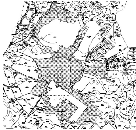
Figure 4 Cadastral plan obtained after GPS survey scale 1:5 000
