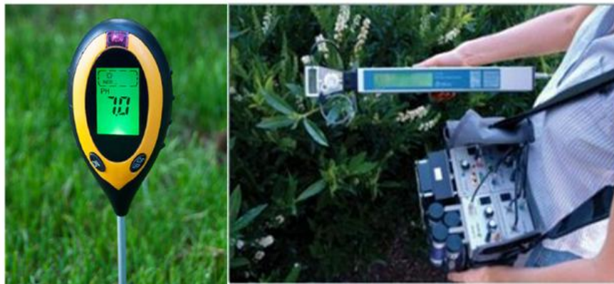
Fig. 4. a) Soil pH and volumetric moisture ratio sensor; b) Sensor for chlorophyll and moisture content in a plant body and/or leaf
