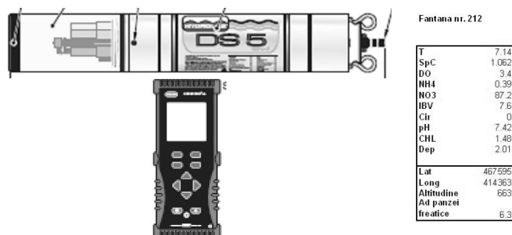
Figure 1. The Hydrolab DS5 Water Quality Multiprobes Sonde and its display
