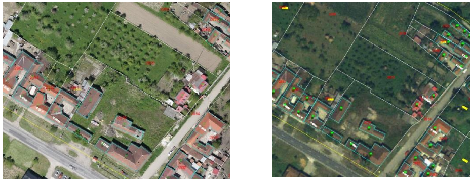
Fig. 8. An orthophotoplan made with Wingtra ONE drone versus an orthophotoplan from the OCPI archive.
