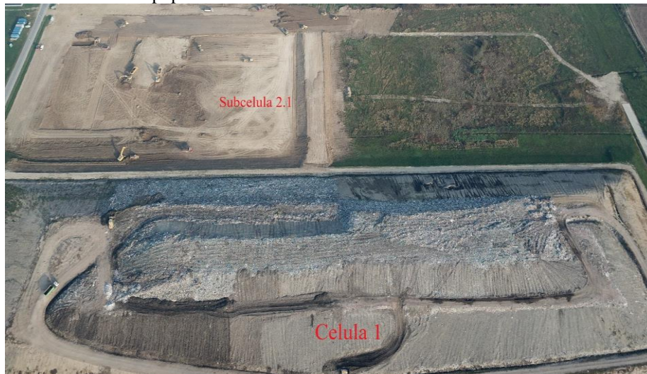
Figure 2. Storage of waste in separate cells Source: S.C. RETIM Ecologic Service S.A.
