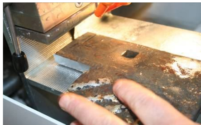
Fig. 3 – Cutting a sample from unhardened zone
