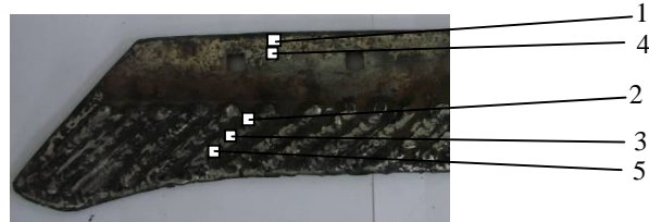
Fig. 1 – Assay areas of the samples 1,4 – not hardened steel samples 2, 3, 5 – bead area samples
