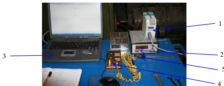
Fig. 6 – Testing stand. Detail with the measurement and control apparatus 1. tensometer amplifier; 2. electronic tachometer with digital display; 3. laptop with acquisition board to measure friction force; 4. digital thermometer; 5. digital calliper rule
