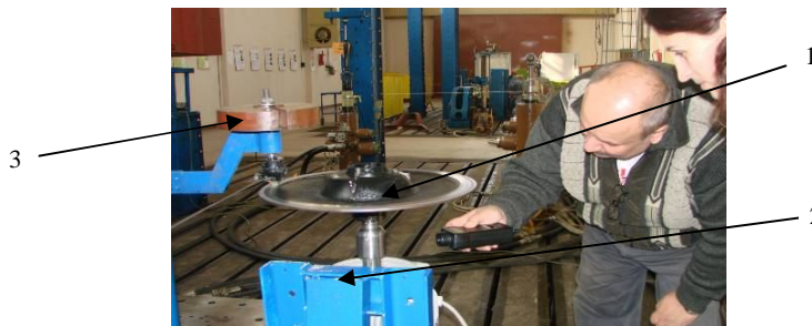
Fig. 5 - Stand for testing samples to friction. Assembly view 1. cast-iron friction disc; 2. engine-disc gear; 3. weights set to realize the pressure
