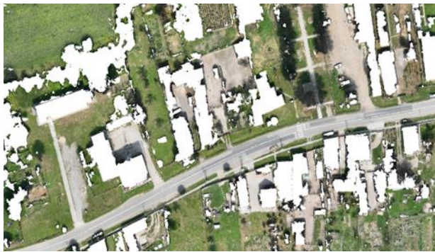
Figure 2. Classified ground points sample
