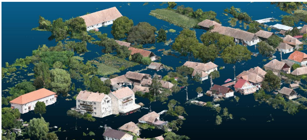
Figure 4. Point cloud sample with the ground points filtered out
