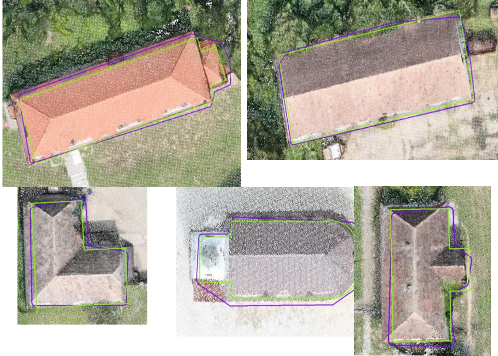
Figure 7. High fidelity outputs, yellow – manually drawn, blue - generated
