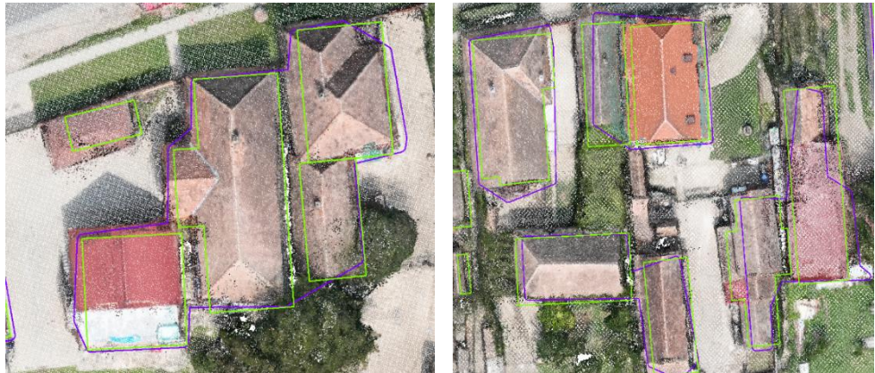
Figure 9. Errors in ouput data, yellow – manually drawn, blue - generated
