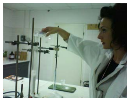
Figure 2. Passing the samples through the florisil column
