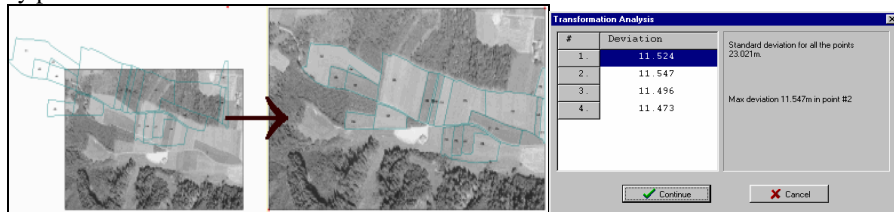
Figure 3. The result of the georeference of a raster image
