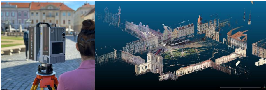
Figure 3. Point cloud result from the terrestrial scanning - CloudCompare view
