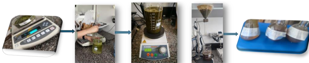
Fig. 2. The steps taken to prepare the extracts (weighing, applying the solvent, stirring the solution, filtering) (photo Ștef Ramona)
