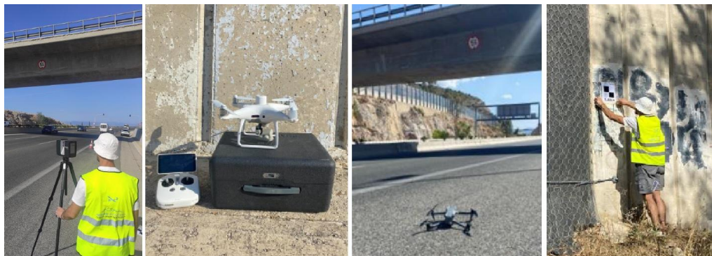
Figure 3. The equipment used during the measurements (a. Faro Focus Premium, b. DJI Phantom 4 RTK, c. DJI Mavic Air 3, d. Checkerboard Targets)
