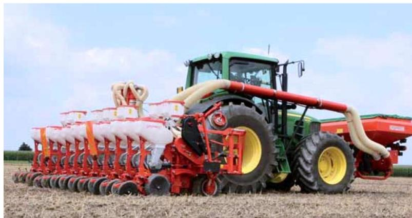
Figure 3: Tractor John Deere 6190R with sowing machine Gaspardo MT 12
