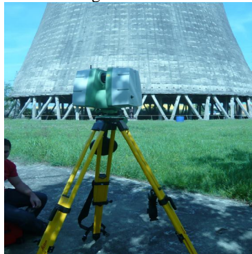
Figure 4: Terrestrial laser scanner
