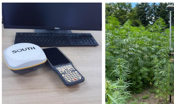
Figure 3 South Galaxy G7 equipment (left) for marking GPS points in the field (right)
