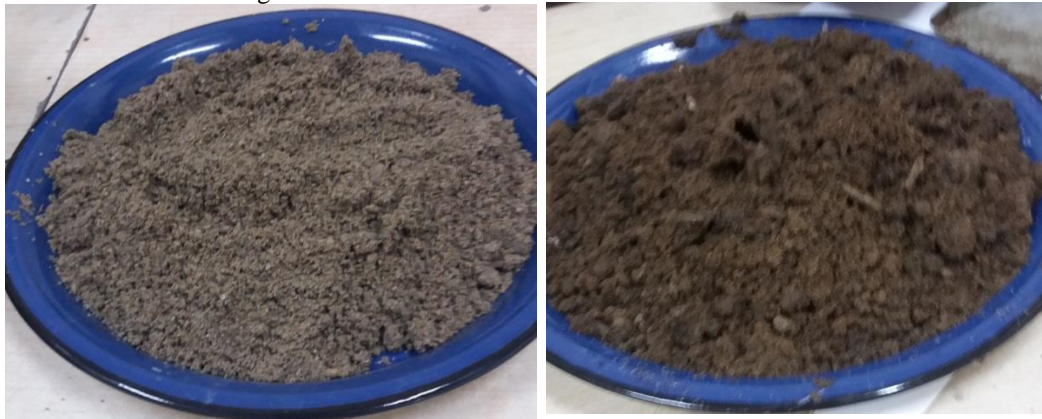
Figure 1. The materials before mixing (sand – left, sludge - right)
