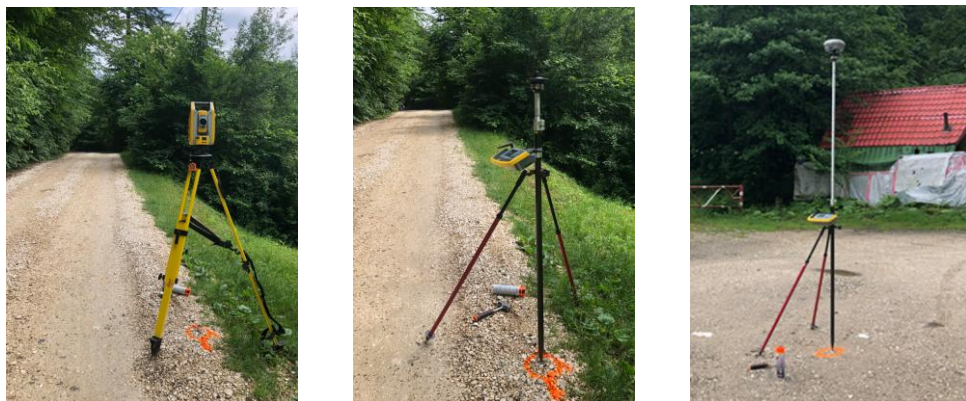
Figure 2. Equipment used: Trimble S5 5'' total station (left); prism pole with 360° prism (centre); prism pole with 360° prism and Trimble R8s GNSS receiver (right).
