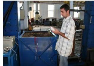
Figure 4 - The tests command centre and the soil humidity measuring with humidometer type HH2
