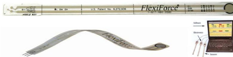
Figure 5 – Force sensor Flexi Force , Laptop and acquisition system
