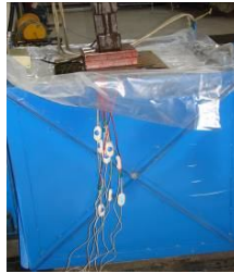
Figure 3- Force sensors applied to the depth of 5÷75 cm with the outputs towards the laptop and the acquisition board
