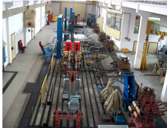
Figure 5 – Testing installation in simulated and accelerated regime type Hydropulse
