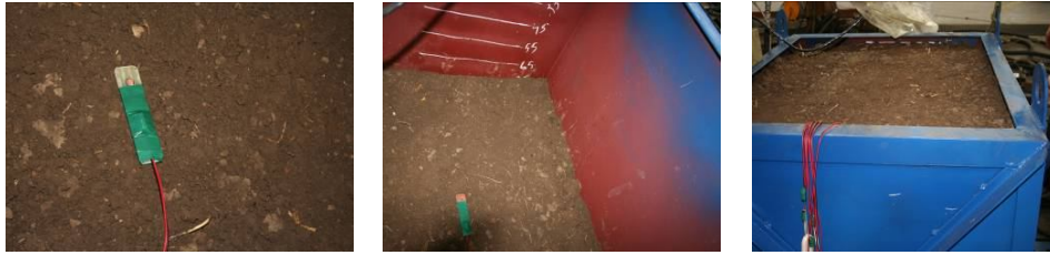
Figure 2 - The force sensor Flexi Force applied on soil before being covered by soil and to the depth of 75 cm and after it was covered to the depth of 5 cm
