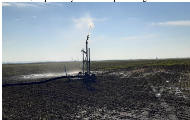
Photo 2 Irrigation system with drum and hose.
