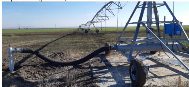
Photo 5 Pivot irrigation system connected to hydrant
