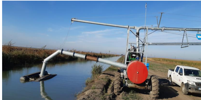
Photo 4 Linear irrigation system with floating pontoon
